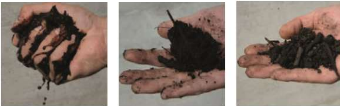
Figure 1.3 Fist test to control the humidity of compost during the composting process. From left to right: too wet, optimal, and too dry
