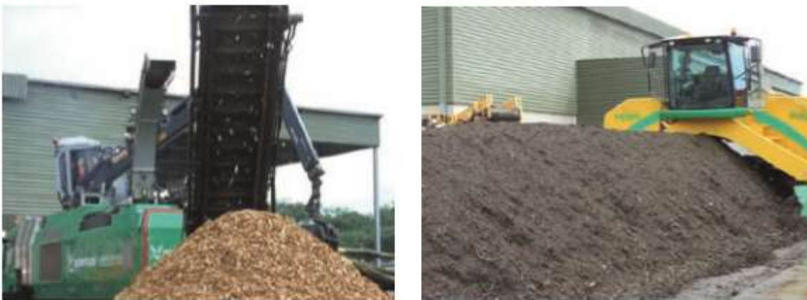
Figure 2.1 Mechanization has made large-scale composting possible: a drum chipper (left) and windrow turner (right).
